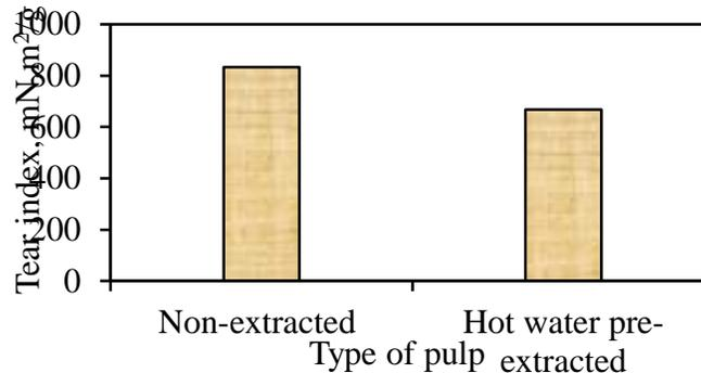
**Fig. 6.** The effect of hot water pre-extraction on tear index in comparison with non-extracted pulp.
