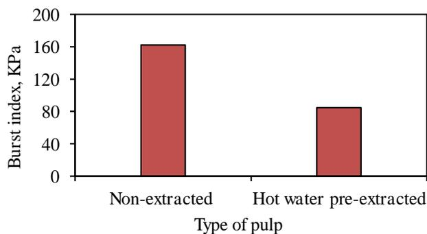
**Fig. 7.** The effect of hot water pre-extraction on burst index in comparison with non-extracted pulp
