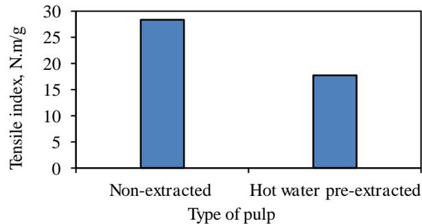
**Fig. 5.** The effect of hot water pre-extraction on tensile index in comparison with non-extracted pulp
