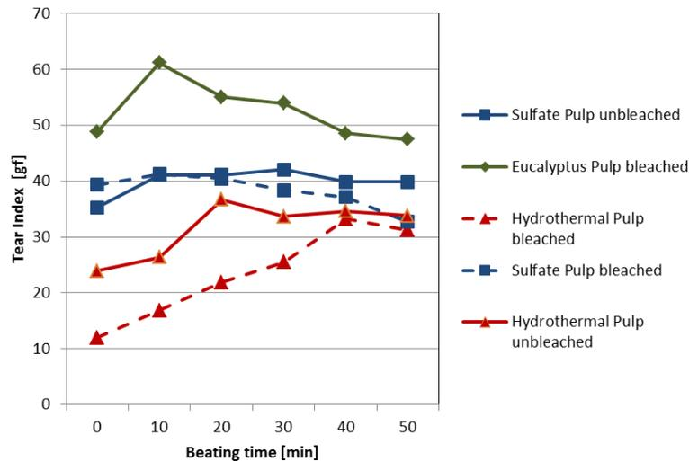
**Fig. 11.** Tear index for bleached pulp
