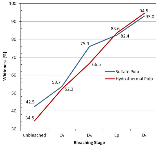
**Fig. 5.** Whiteness value for O<sub>2</sub>D<sub>0</sub>E<sub>P</sub>D<sub>1</sub> bleaching sequence
