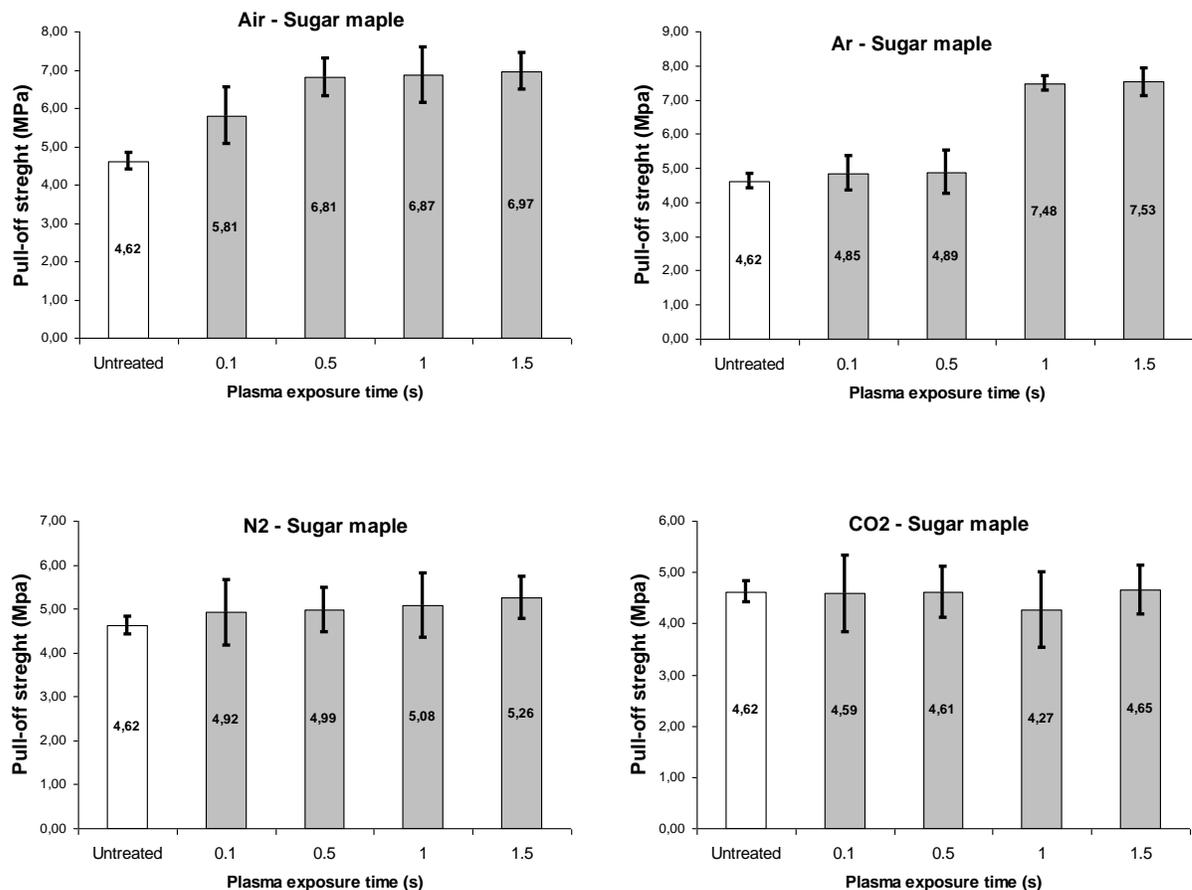
**Fig. 7.** Sugar maple pull-off strength as a function of plasma exposure time
