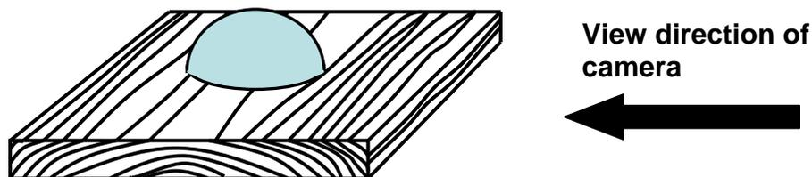
**Fig. 2.** View direction of camera with respect to the wood grain
