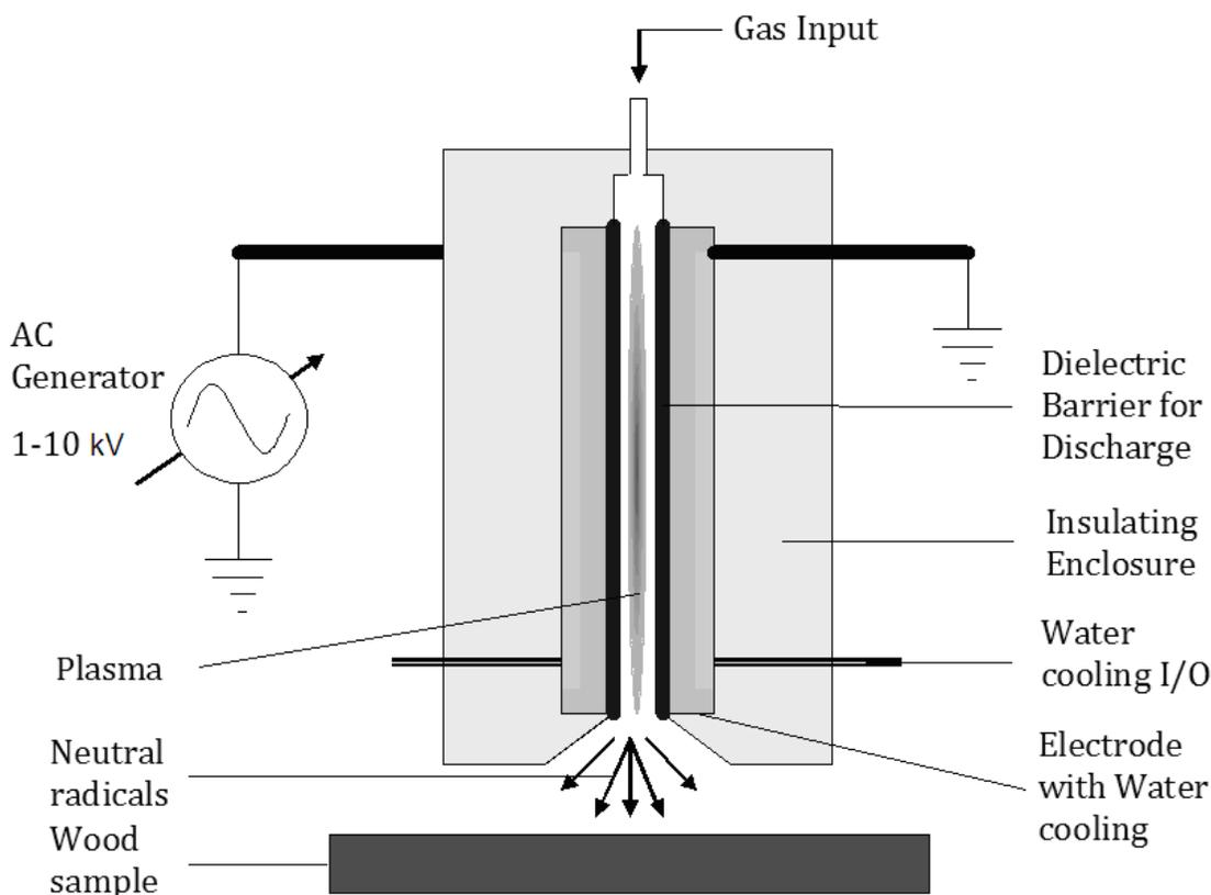
**Fig. 1.** Schematics of the flowing DBD apparatus used in this work - wood samples are moved on a conveyer along the plasma jet
