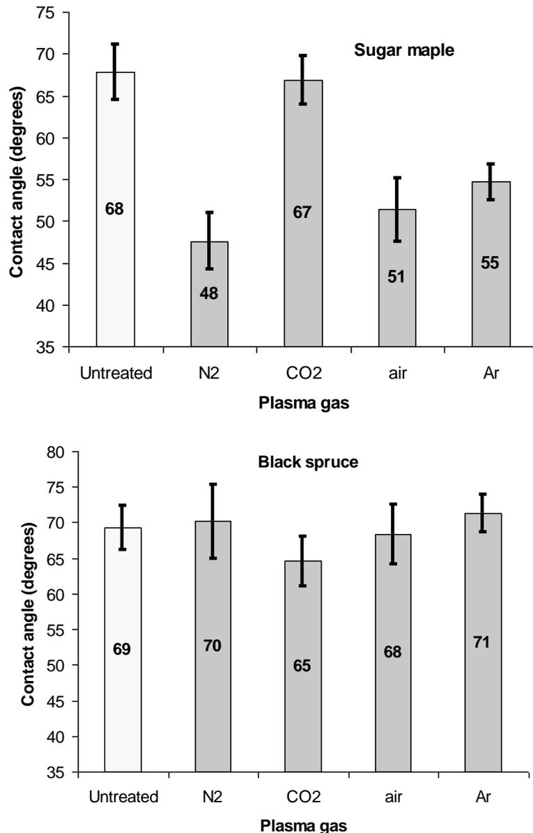
**Fig. 3.** Influence of plasma gas on wettability with water of sugar maple (top) and black spruce (bottom) for a plasma exposure time of 1.5 s
