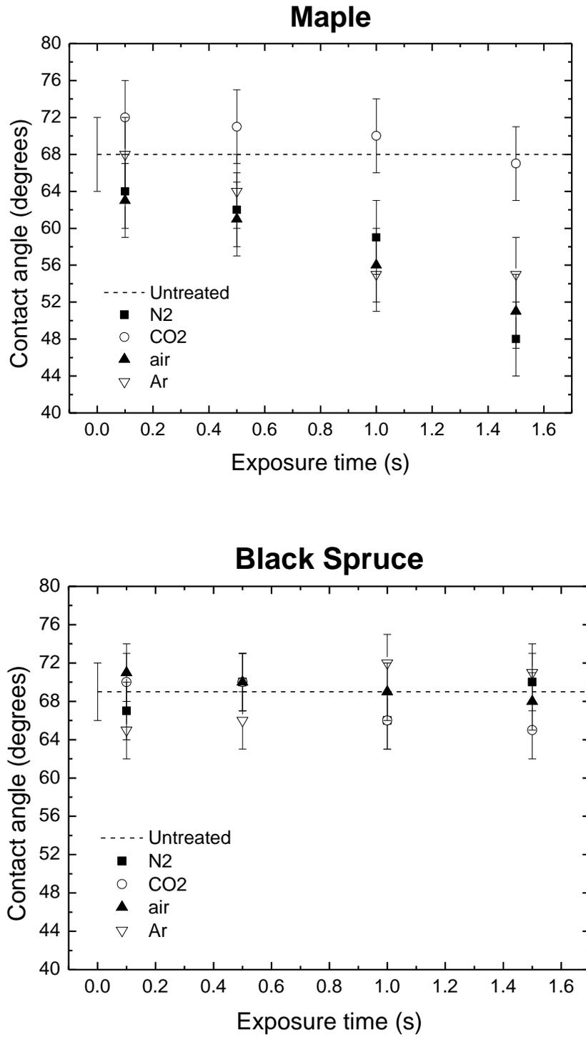
**Fig. 4.** Mean contact angle of water as a function of plasma exposure time for sugar maple (top) and black spruce (bottom). Dotted lines represent values for control samples.
