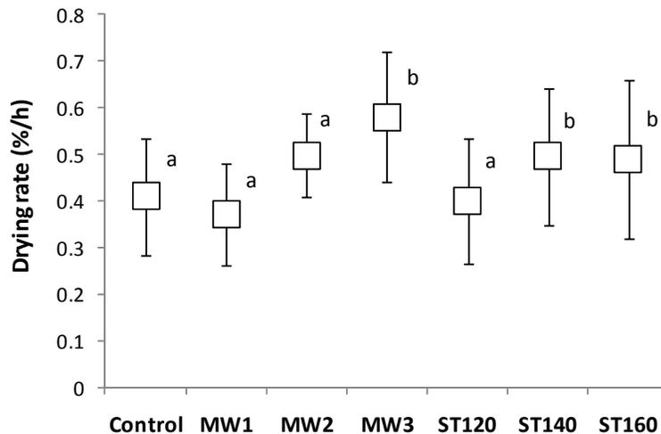
**Fig. 2.** Drying rate of microwave and steam exposed fir wood specimens compared to the unexposed ones
