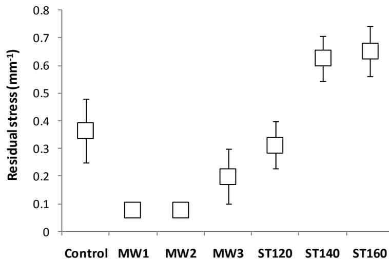
**Fig. 3.** Intensity of residual drying stresses in microwave and steam exposed fir wood specimens compared to the unexposed ones
