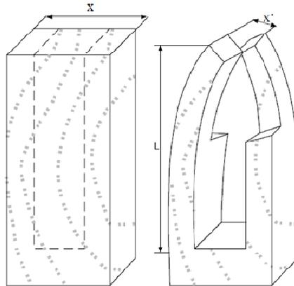
Fig. 1. Cutting method of specimens for measurement of casehardening (internal residual stresses)
