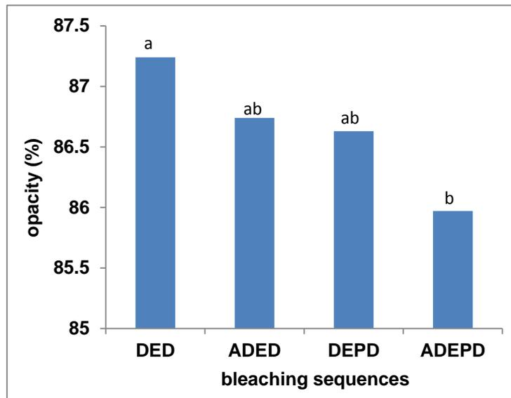
**Fig. 8.** The effect of acid pretreatment and peroxide reinforcement in alkaline extraction stage in DED bleaching on paper opacity
