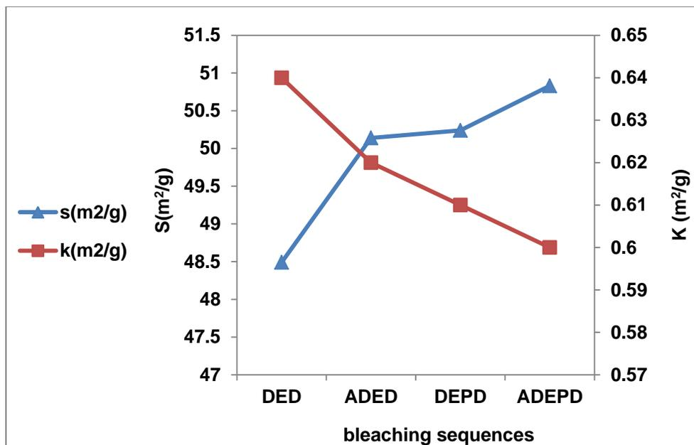
**Fig. 9.** The effect of acid pretreatment and peroxide reinforcement in alkaline extraction stage in DED bleaching on light scattering and absorption coefficients of paper
