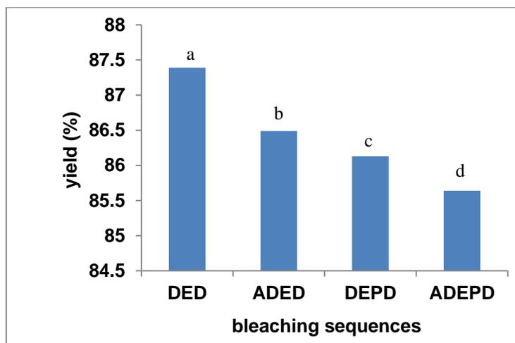
**Fig. 2.** The effect of acid pretreatment and peroxide reinforcement in alkaline extraction stage on the final pulp yield of DED bleached pulp (based on OD chips)
