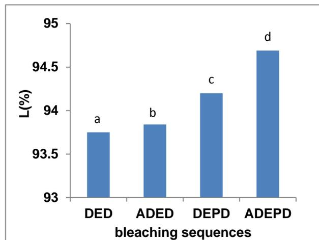
**Fig. 5.** The effect of acid pretreatment and peroxide reinforcement in alkaline extraction stage on the *L* factor of DED bleached pulp
