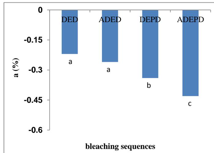
**Fig. 6.** The effect of acid pretreatment and peroxide reinforcement in alkaline extraction stage on the *a* factor of DED bleached pulp
