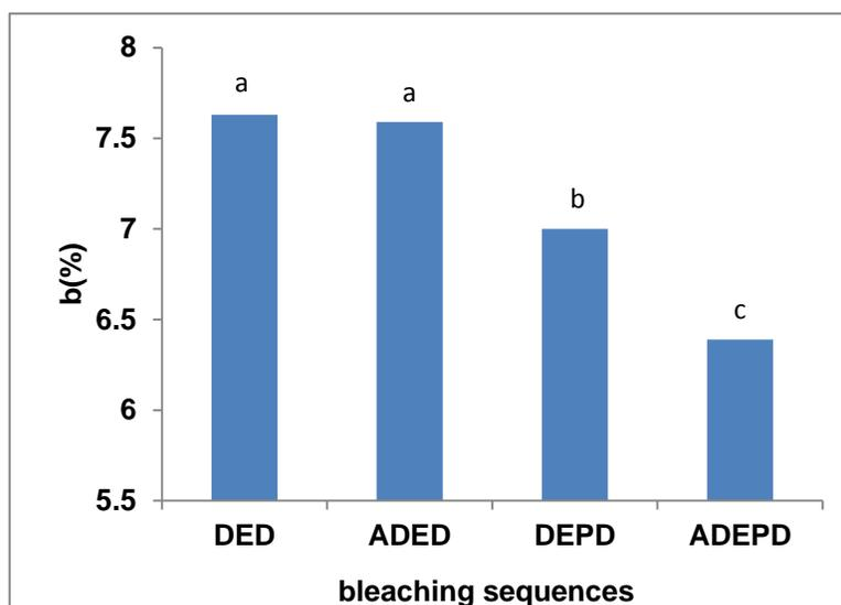
**Fig. 7.** The effect of acid pretreatment and peroxide reinforcement in alkaline extraction stage on the *b* factor of DED bleached pulp
