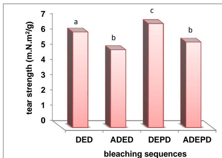
**Fig. 14.** The effect of acid pretreatment and peroxide reinforcement in alkaline extraction stage in DED bleaching on tear strength of paper
