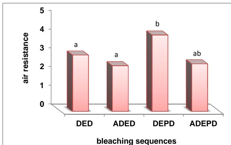
**Fig. 11.** The effect of acid pretreatment and peroxide reinforcement in alkaline extraction stage in DED bleaching on air resistance of paper
