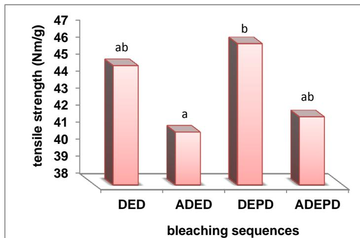
**Fig. 12.** The effect of acid pretreatment and peroxide reinforcement in alkaline extraction stage in DED bleaching on tensile strength of paper
