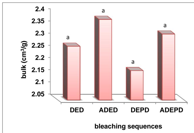
**Fig. 10.** The effect of acid pretreatment and peroxide reinforcement in alkaline extraction stage in DED bleaching on bulk of paper
