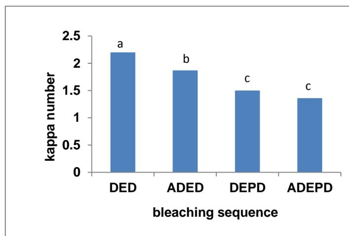
**Fig. 1.** Effect of acid pretreatment and peroxide reinforcement in alkaline extraction stage on the final kappa number of DED bleached pulp
