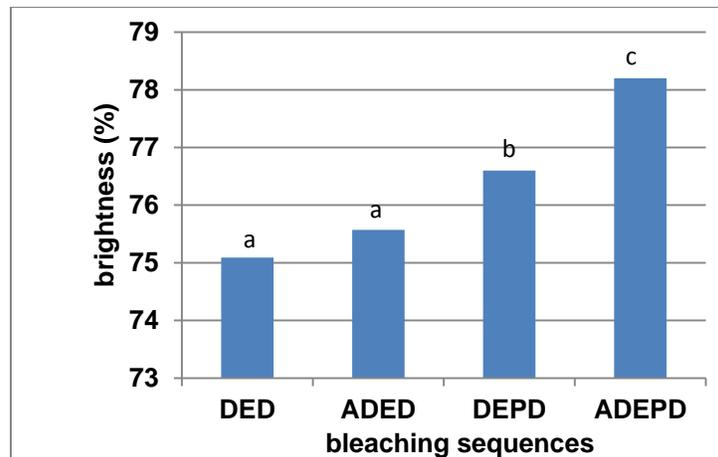
**Fig. 3.** The effect of acid pretreatment and peroxide reinforcement in alkaline extraction stage on the final pulp brightness of DED bleached pulp
