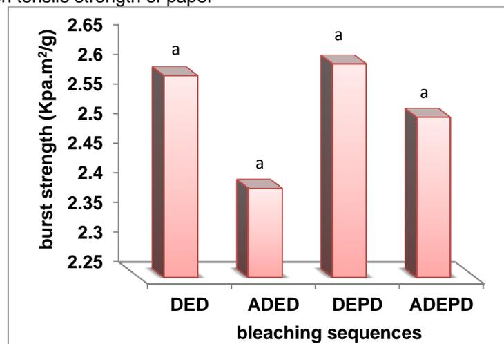
**Fig. 13.** The effect of acid pretreatment and peroxide reinforcement in alkaline extraction stage in DED bleaching on burst strength of paper
