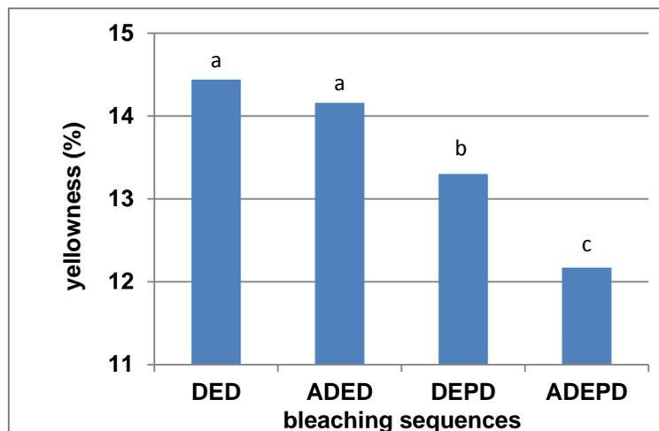
**Fig. 4.** The effect of acid pretreatment and peroxide reinforcement in alkaline extraction stage on the final pulp yellowness of DED bleached pulp
