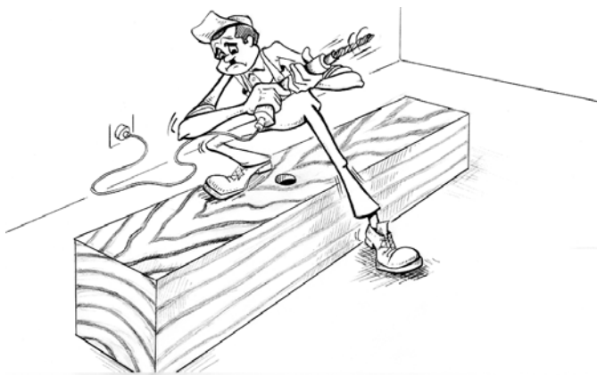
Fig. 1. Drilling a hole at the middle of the beams on the tangential surface in radial direction.
