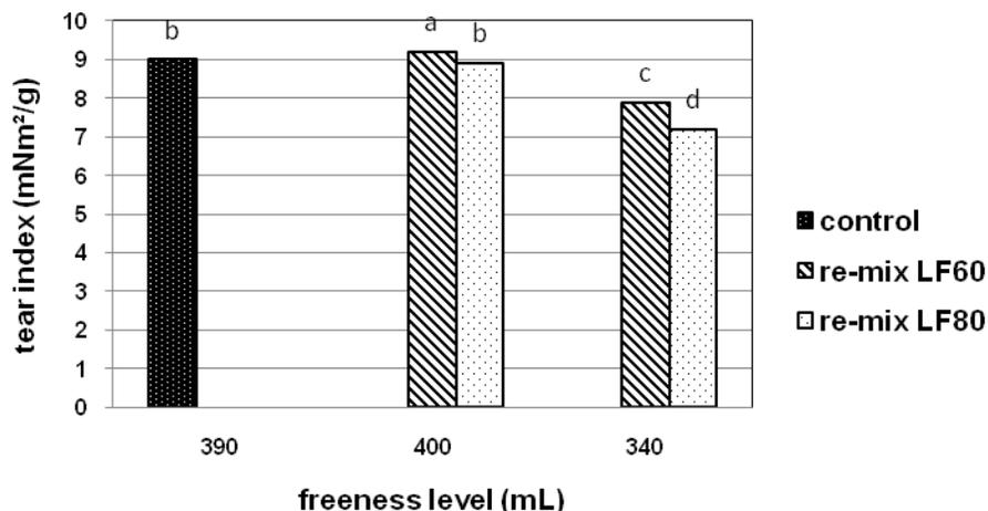
**Fig. 6.** Effect of fiber fractionation and refining degree on tear index
