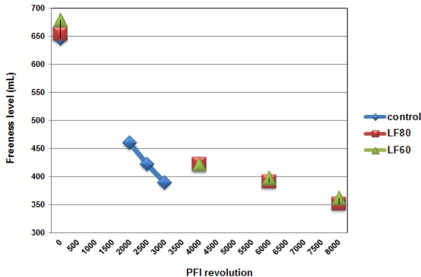
**Fig. 2.** Refining response of fractionated long fiber samples versus unfractionated control pulp
