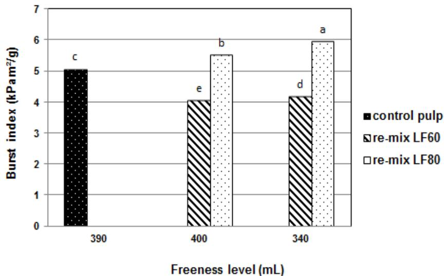
**Fig.5.** Effect of fiber fractionation and refining degree on burst index
