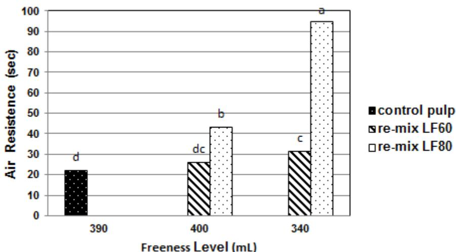
**Fig. 3.** Effect of fiber fractionation and refining degree on air resistance of paper
