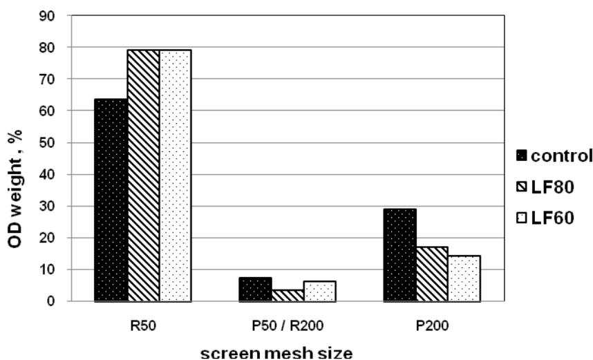
**Fig. 1.** Fiber distribution of unrefined long fiber fraction samples as compared to the unrefined control straw pulp
