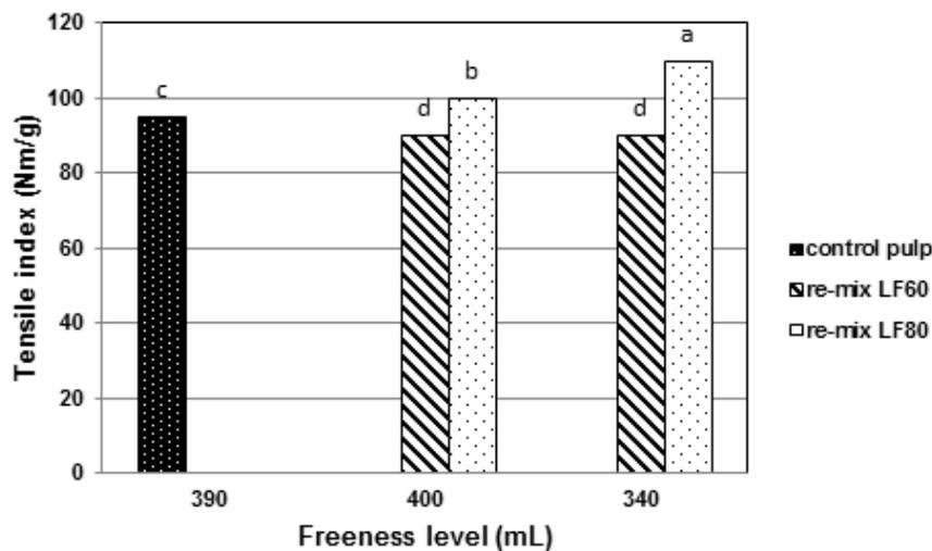
**Fig.4.** Effect of fiber fractionation and refining degree on tensile index
