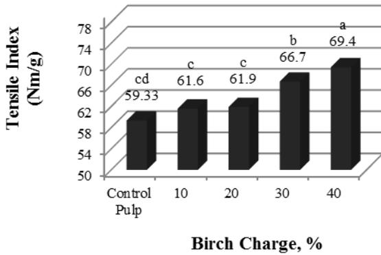
**Fig.6.** The effect of different charges of birch on pulp tensile index.
