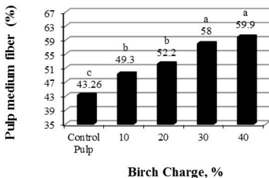
Fig.3. The effect of different charges of birch on pulp medium fiber fraction.
