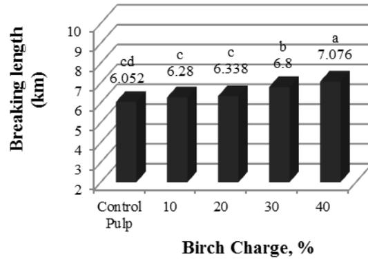
**Fig.7.** The effect of different charges of birch on pulp breaking length.
