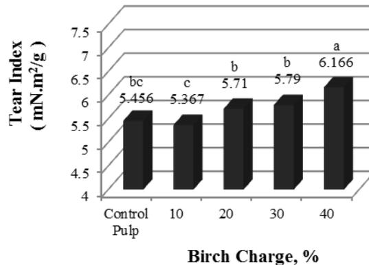
**Fig.9.** The effect of different charges of birch on pulp tear index.
