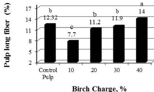
Fig2. The effect of different charges of birch on pulp long fiber fraction.
