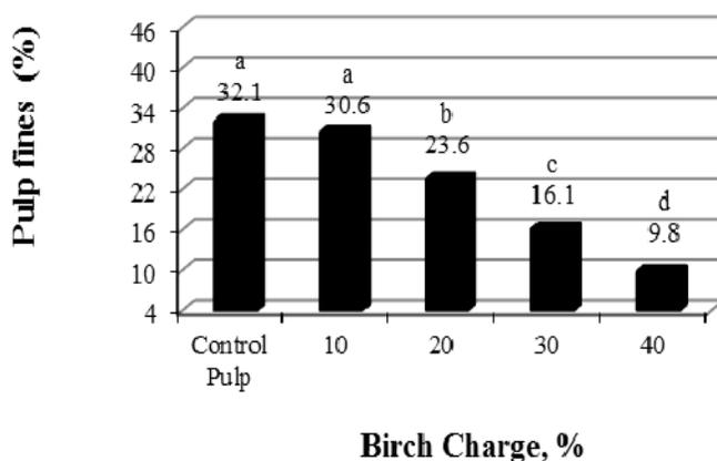
**Fig.5.** The effect of different charges of birch on pulp fine content.
