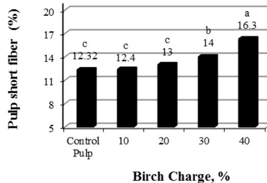
Fig.4. The effect of different charges of birch on pulp short fiber fraction.
