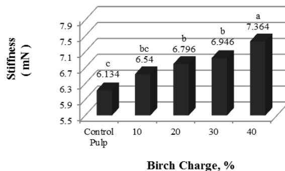
**Fig.10.** The effect of different charges of birch on pulp stiffness.
