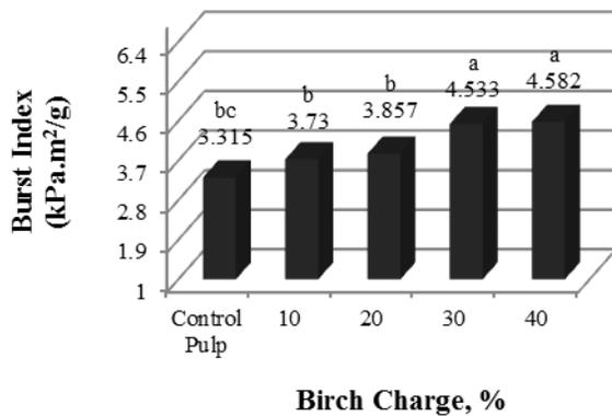
**Fig.8.** The effect of different charges of birch on pulp burst index.
