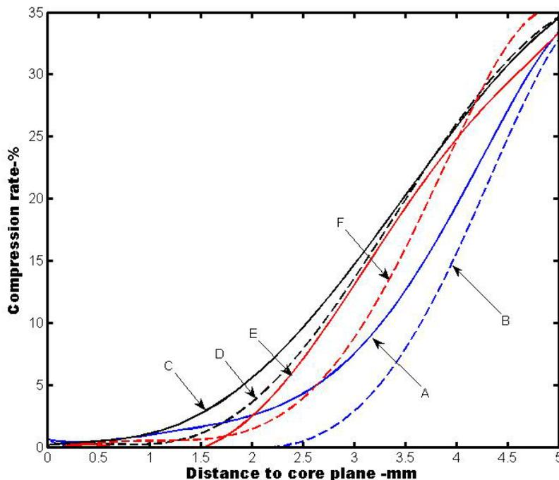
**Fig. 2.** Compression rate as a function of the distance to core plane in half thickness of specimens
