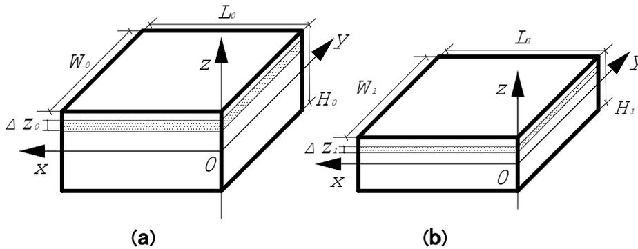
**Fig.1** Schematic diagrams of wood specimens before (a) and after (b) densification
