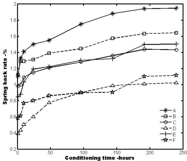
**Fig. 3.** Spring-back rate after conditioning at room temperature of densified poplar wood specimens
