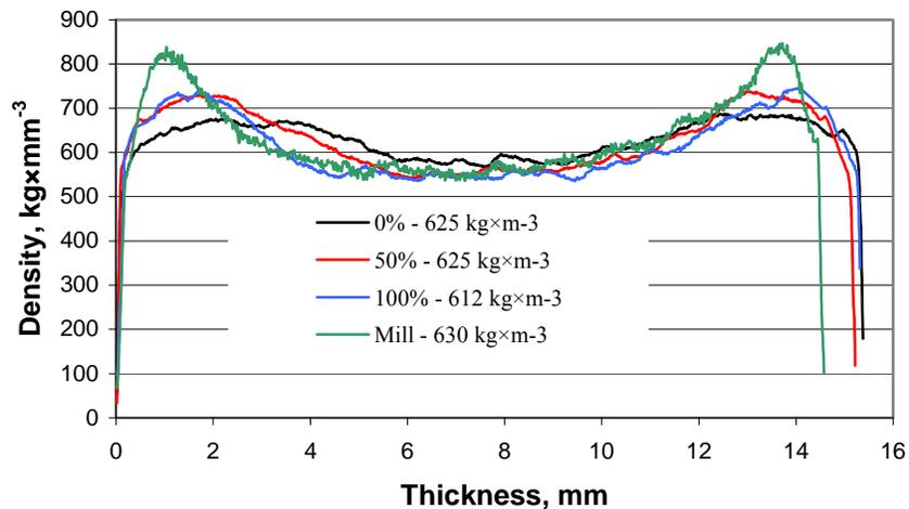
**Fig. 9.** Vertical density profiles of OSB board glued with pMDI
