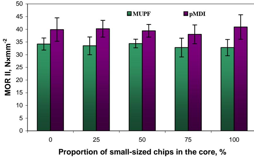
**Fig. 2.** Bending strength of OSB determined for the longer axis
