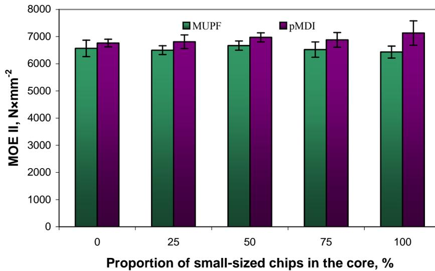
**Fig. 3.** Modulus of elasticity of manufactured OSB determined for the longer axis
