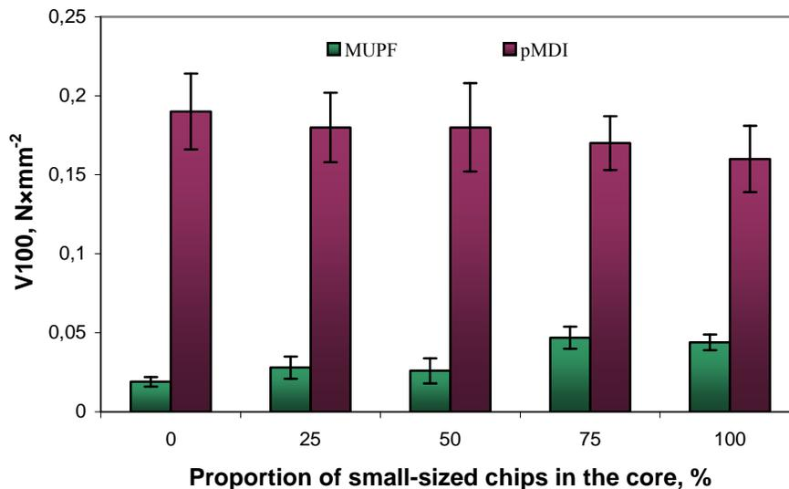
**Fig. 7.** Internal bond of manufactured OSB after the boiling test
