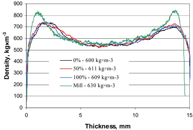
**Fig. 8.** Vertical density profiles of OSB board glued with MUPF resin
