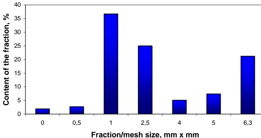
Fig. 1. Sieve fraction of particleboard chips
