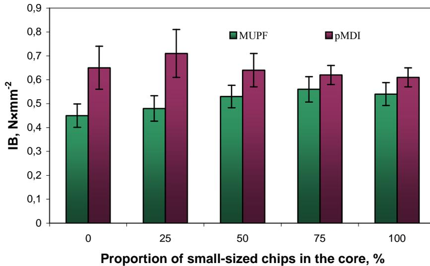
**Fig. 6.** Internal bond of manufactured OSB
